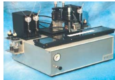
XYZ3050 Configured with 2 BioJet Quanti and 1 AirJet Quanti Dispenser
