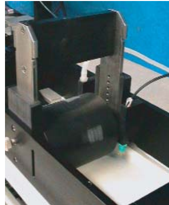
Dip Tanks with Liquid Level Sensor
